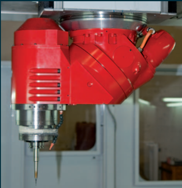
Universal milling head with high speed spindle
