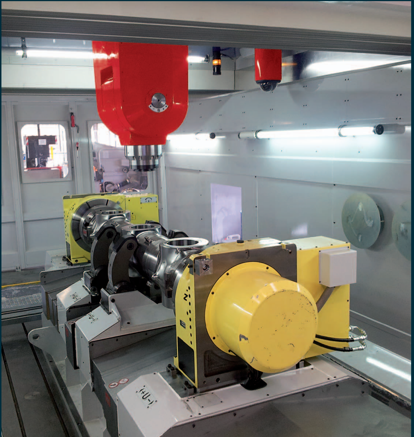
5-axis machining of a titan landing gear for aerospace industry
