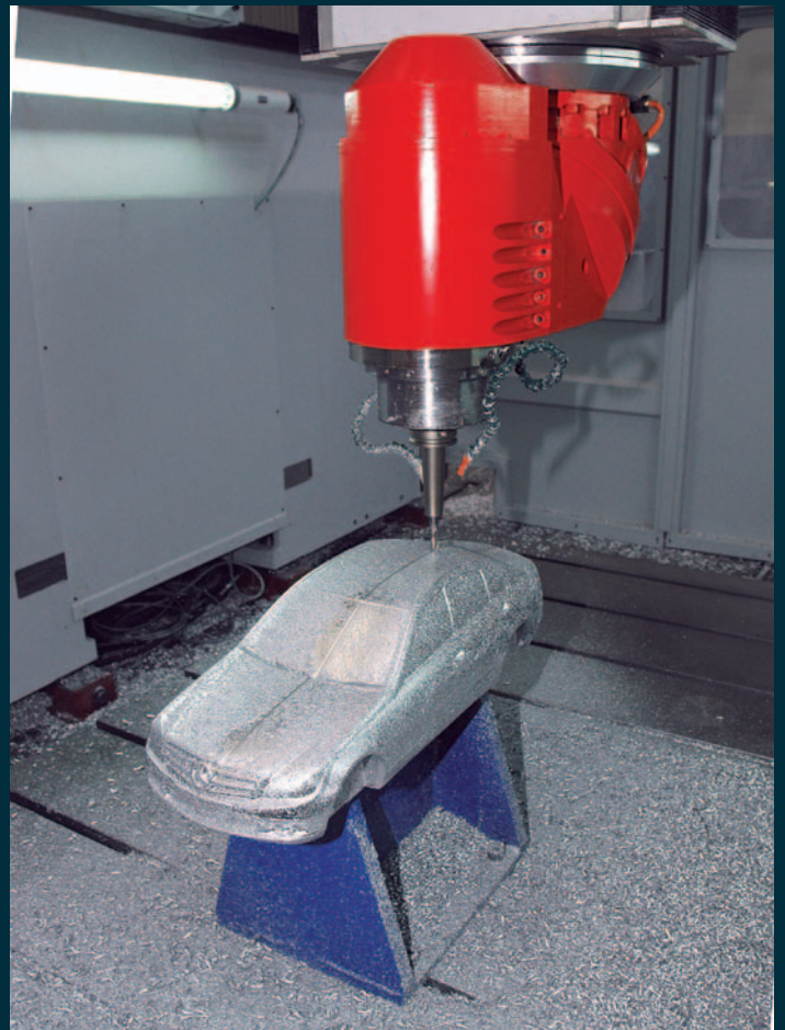
High speed machining of an aluminium car model
