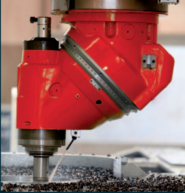
Universal milling head with automatic millesimal positioning
