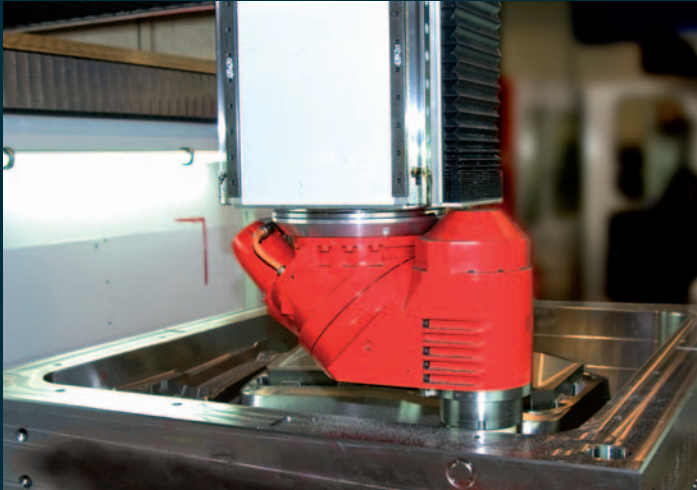
Machining of a plastic injections mould for automotive industry
